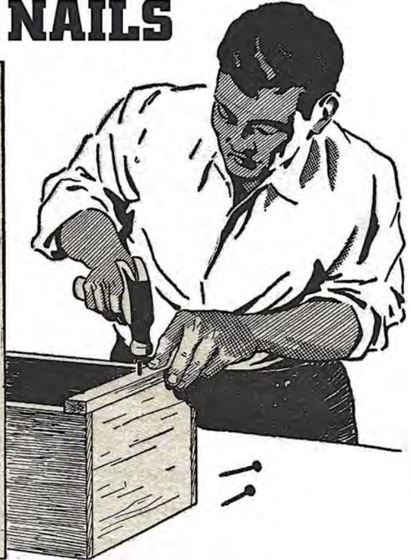
Don't hammer like the workman above. He's holding the hammer too close to the head and has his left index finger in a dangerous spot. Note how grain lined nails have wood in Fig. 1. Angle driven nails in Fig. 2 hold better.
