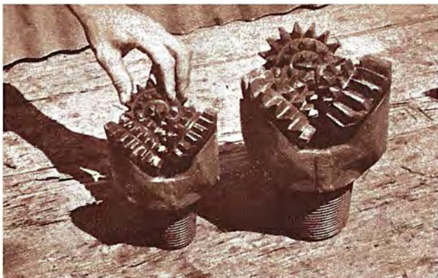
Above are rock bits, revolving grinders that are used when the going gets tough for the drill.
