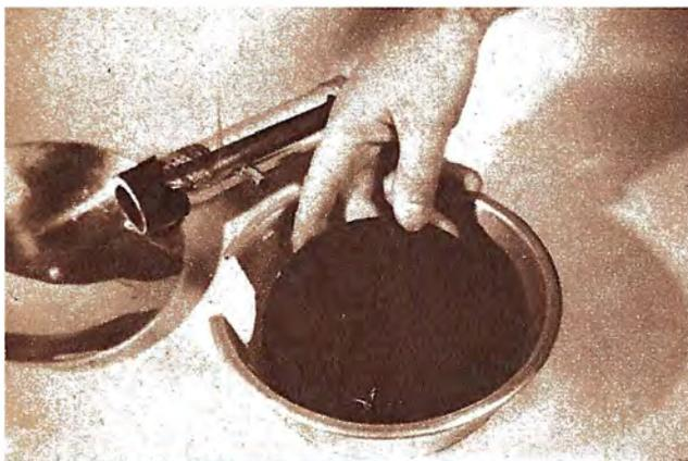
ABOVE: Fitting the filter disc into the cut-out bottom of the pan. Slight indentations in the pan hold it in place. RIGHT: The improvised flashfilter unit is held to the standard flash reflector by means of indentations pressed into the side of the aluminum pan. The unit may be snapped loose quickly for changing of flash bulbs between exposures.
