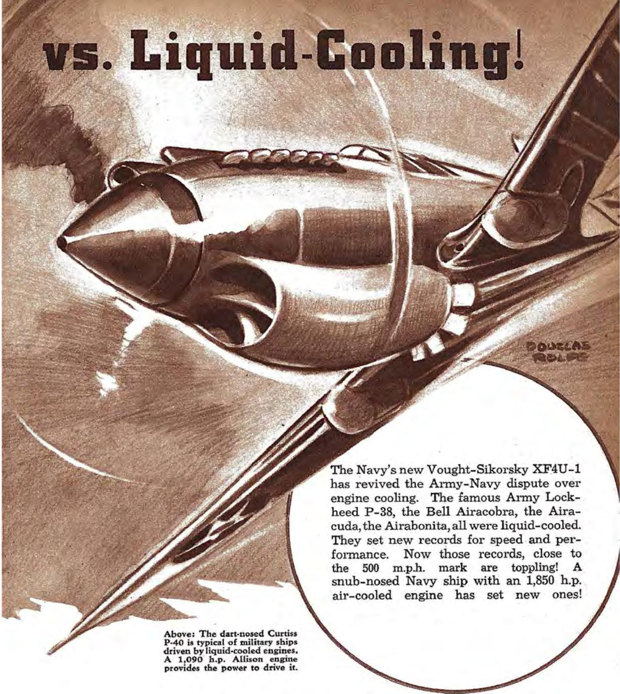
Above: The dart-nosed Curtiss P-40 is typical of military ships driven by liquid-cooled engines. A 1,090 h.p. Allison engine provides the power to drive it.
