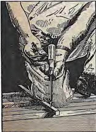
WHEN driving screws in hard wood, a hole bored through the handle of the screwdriver as shown, will be a great help. A large nail can be inserted through the hole to act as a lever, when desired.—A. V.
