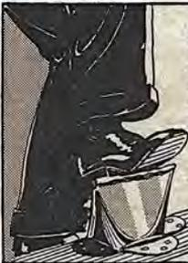
SQUEEZE TOP IN AND BEND OVER FOR A TIGHT SEAM
