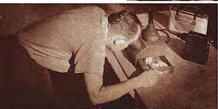
Rock specimens may be viewed in daylight by putting them into a drawer in this cabinet, shoving it under ultraviolet torch which plugs into the top, and looking down through the peephole. Such equipment is very useful in field work either by day or by night.
